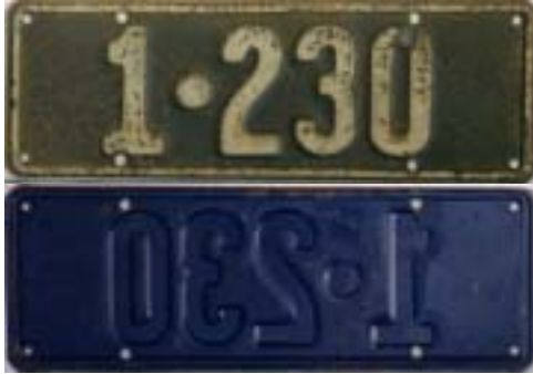
This shows how defectively the front of a plate usually withstood the elements in comparison to the back.
